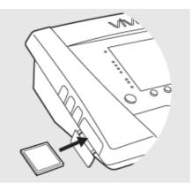
2.When the memory card is inserted into the ventilator the Device Memory menu is automatically displayed. Choose Save
