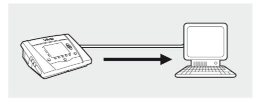
For electrical safety reasons it is recommended to use a laptop running on battery, not connected to mains. Using a desktop or laptop PC connected to mains may require an isolated USB cable, depending on the symbol of the ventilator's USB port:
