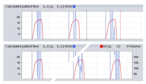
Some views contain data graphs over registred data. Each graph may contain one or two types of data. In the cases with two types of data different colours are used for the graphs and the vertical axis on the right and left sides respectively represent the two types of data.
