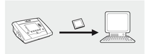
**1.** Insert the memory card in the memory card slot on the side of the Vivo 50/60. Make sure the memory card is properly inserted.
